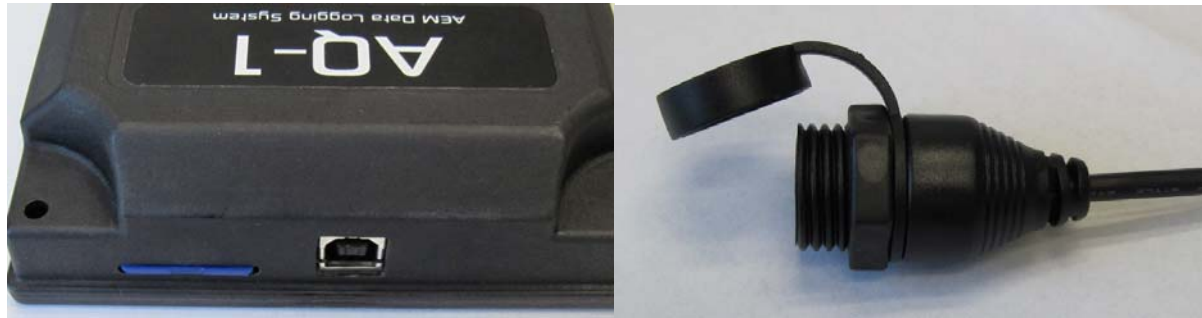
Figure 6. AQ1 On-Board (Left) and Harness (Right) USB Ports
